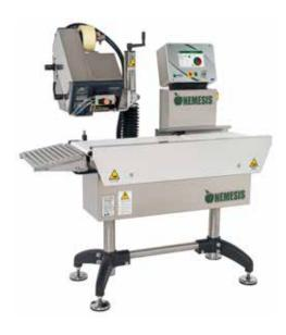
speed of 30 m/min. The software was so configurated as **not to label under- and overweight products** with respect to the compliance values set up by the machine operator, thus meeting the original request of easily differentiating non-compliant trays.
